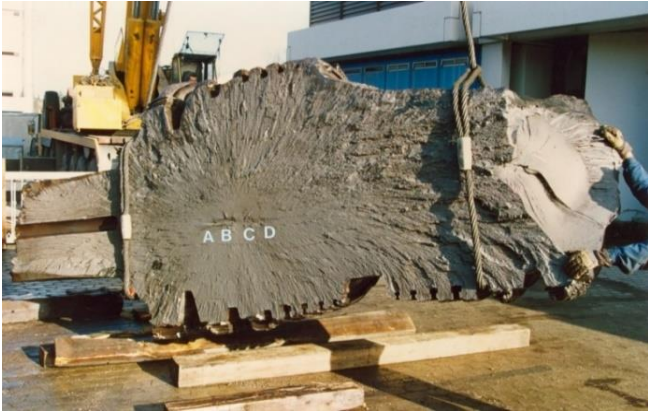
Fig. 10: Brittle fracture of the turbine shaft
