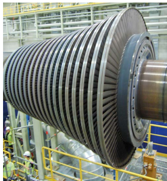
Steam turbine before installation
