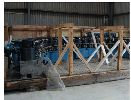
Insufficient preservation of the machine parts in a wooden box without dry air preservation
