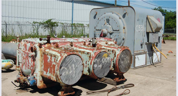
Corrosion due to storage of a compressor in an open air area without sufficient protection
