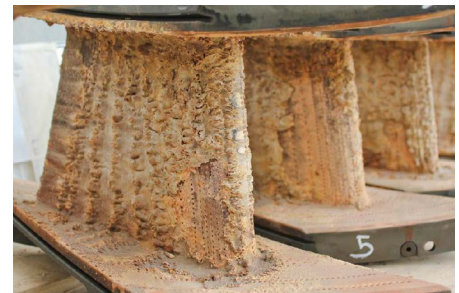
GT Row 1 Vanes with deposits due to sand ingress
