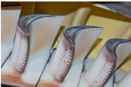
Row 1 Turbine Blades with tip rubbing
