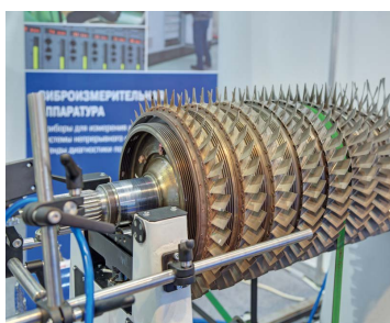
Low speed balancing of compressor rotor
