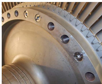
Steam turbine before installation
